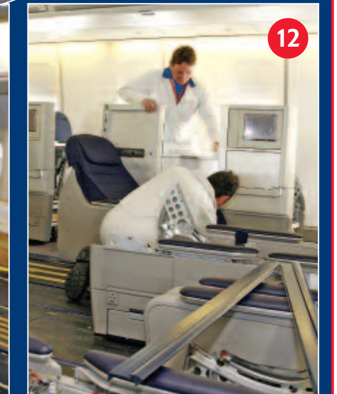
Fitting the seats in a tight space
