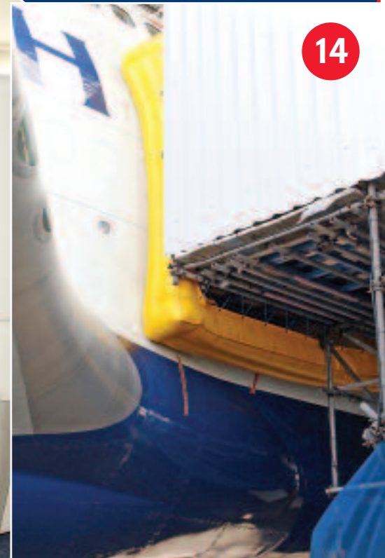
The bouncy castle used to seal the plane during fitting
