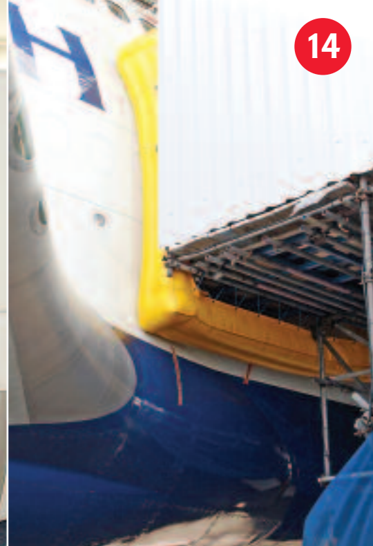
The bouncy castle used to seal the plane during fitting
