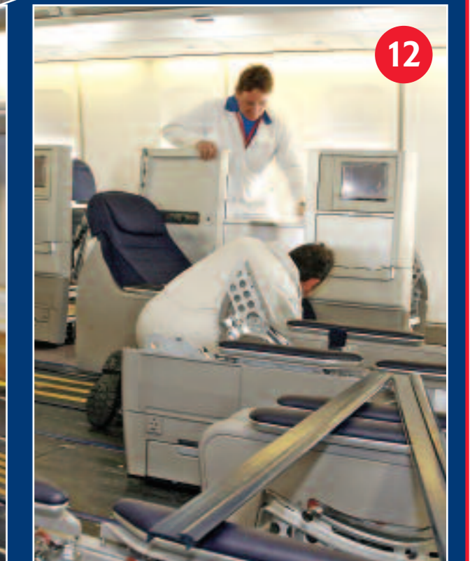
Fitting the seats in a tight space
